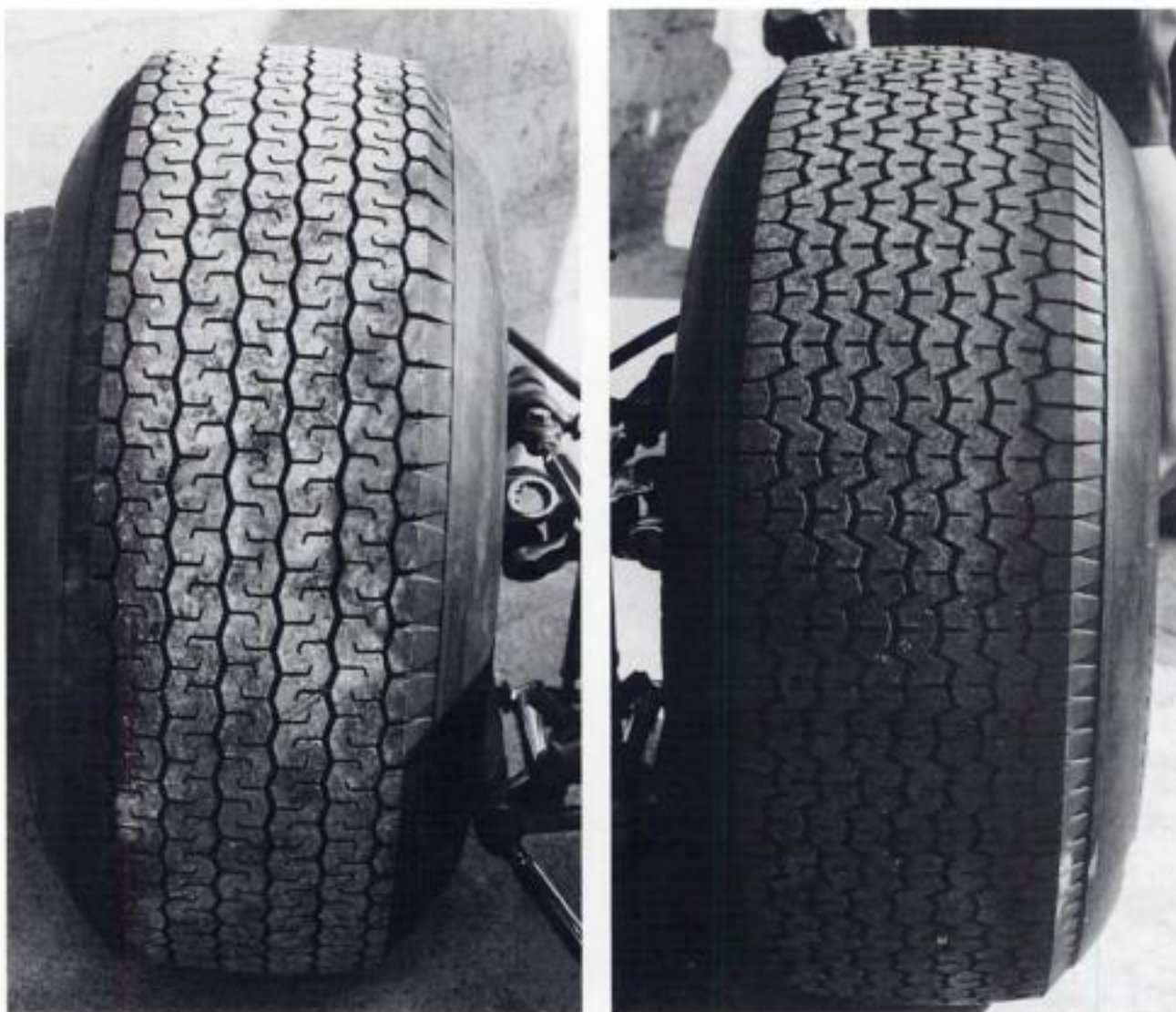
The first skirmishes in what will become a tyre war in the later '60s – the Dunlop R7 tread pattern for 1965 (left) and the Goodyear WA type reply (right).
